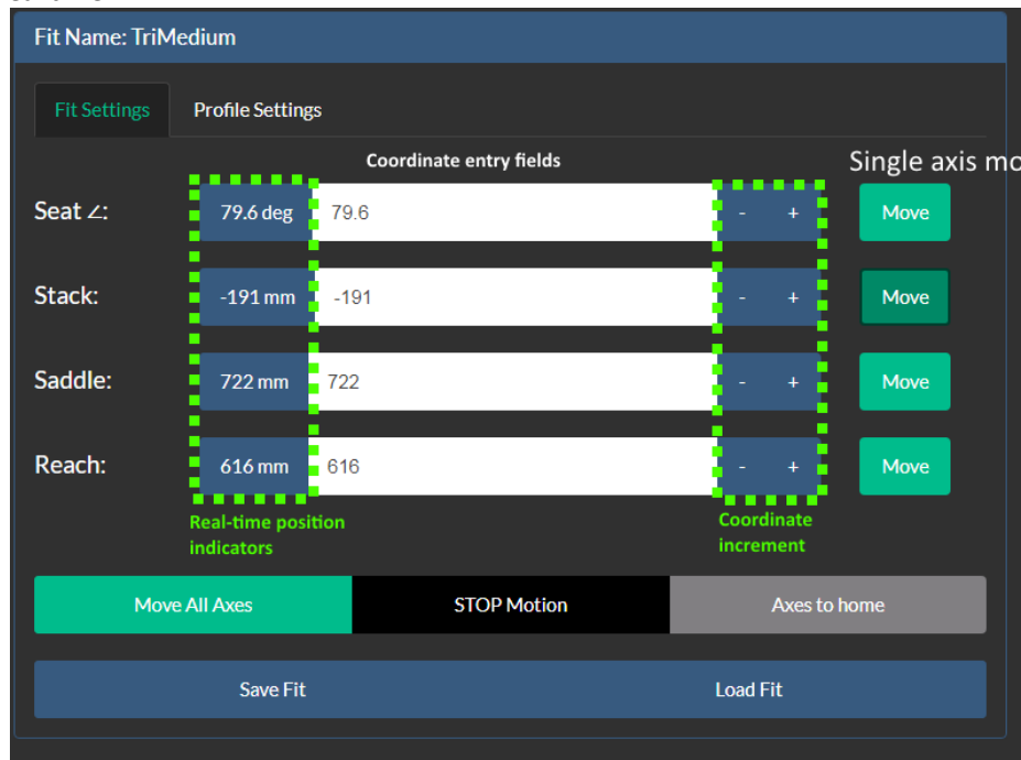
Figure 8: Vertex Fit UI axis movement controls. Coordinates may be typed in or incremented via the +- buttons. Clicking or touching any of the move buttons activates the Vertex. Position indicators show the position of each axis in real time.
